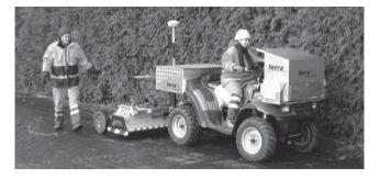
Figure 1: Mounting of the used stepped-frequency GPR array on a Quad bike.
